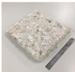
(a) Feather fibre fabric, density 29.8 kg/m 3
