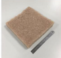
(i) PET fabric, density 25.5 kg/m 3
