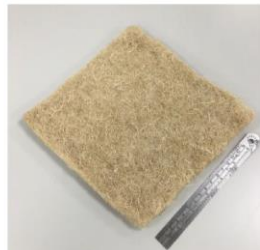
(c) Hemp fabric, density 83.3 kg/m 3
